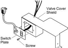
Figure 19 - Installing Switch Plate to Valve Cover Shield
